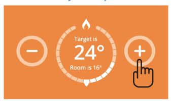
To INCREASE the room temperature, repeatedly press the •• button on the Switchee until your target temperature is displayed centrally. The flame icon/symbol will be highlighted when the Heating is turned ON.
