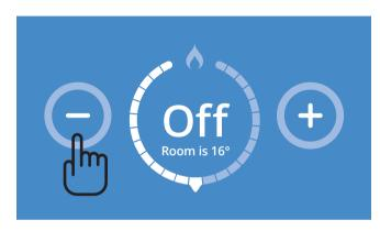
Repeatedly press the minus button on the Switchee until the Target temperature (large number displayed centrally) is below the room's actual temperature (smaller number displayed below the target temperature).
