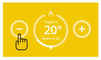
To DECREASE the room temperature, repeatedly press the button on the Switchee until your target temperature is displayed centrally.
